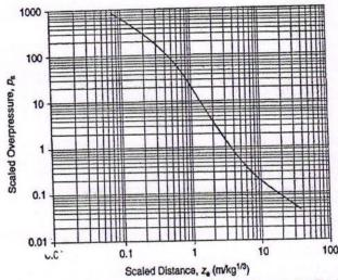
One Thousand kilogram of methane escapes from a storage vessel, mixes with air, and explodes. Determine (a) The equivalent amount of TNT and (b) the side on peak overpressure at a distance 50 m from the blast. Assume an explosion efficiency of 2 %.  $\Delta H_c$  for Methane is 802.3 kJ/mol and the energy of explosion of TNT is 4686 kJ/kg.
